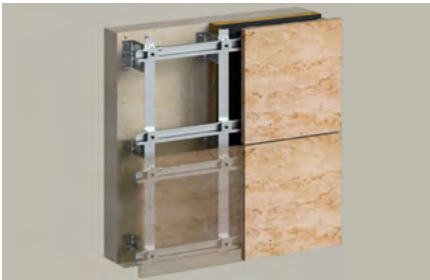
System illustration FLH-R with ATK100 + 103 and FZP II in natural stone
